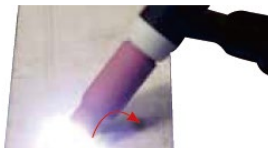
(18) Now rotate the Gas Cup in the reverse direction to lift the Tungsten electrode from the work piece to create the arc.
