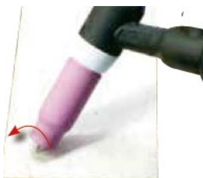
(17) With a small movement rotate the gas cup forward so that the tungsten electrode touches the work piece.
