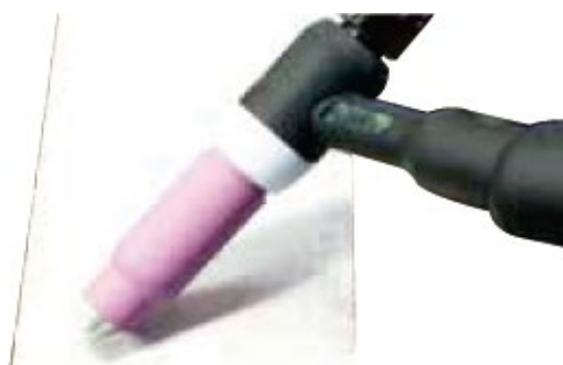
(16) Lay the outside edge of the cup on work piece with the tungsten Electrode 1-2mm from the work piece. Press and hold the trigger button on TIG torch to start the gas flow.
