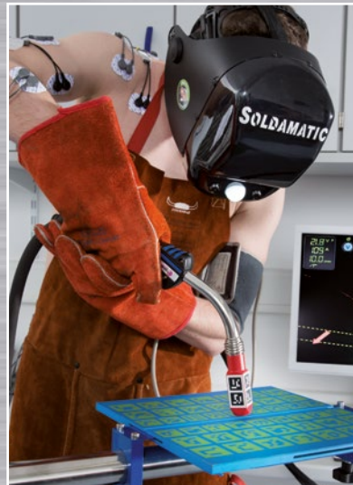
MB EVO PRO 36 in welding position PA (horizontal welding of butt and fillet welds).
