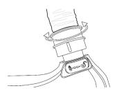
3) Connect the other end of the tube to the headgear in the same way.
