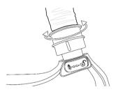
2) Insert the airflow tester at the top of the tube.
