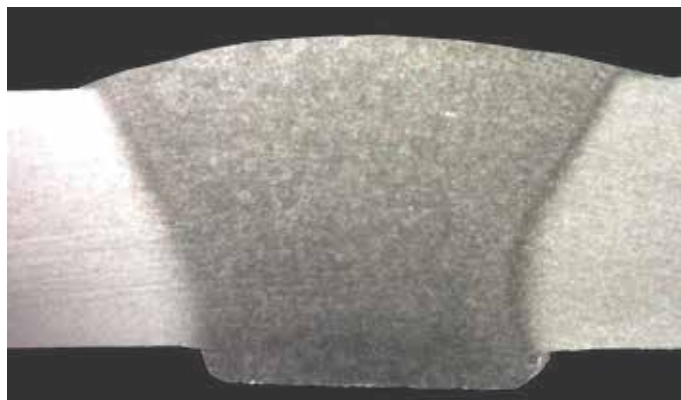
1 Pass - 1.6 mm 5356 - approximately 22 ipm travel speed 23.0 V; 342 ipm wire feed speed
