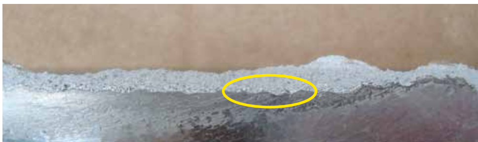
When complete fusion is achieved, the edge of the vertical component will be melted away by the weld metal.
