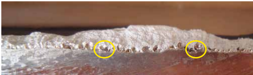
Porosity will show up as very shiny, spherical inclusions.
